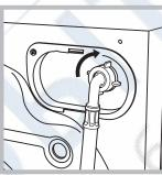
2. Connect the inlet hose to the washing machine by screwing it onto the corresponding water inlet of the appliance, which is situated on the top right-hand side of the rear part of the appliance (see figure).
